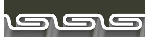
Interlocked Design 1-1/2" through 4" with no bonding wire
